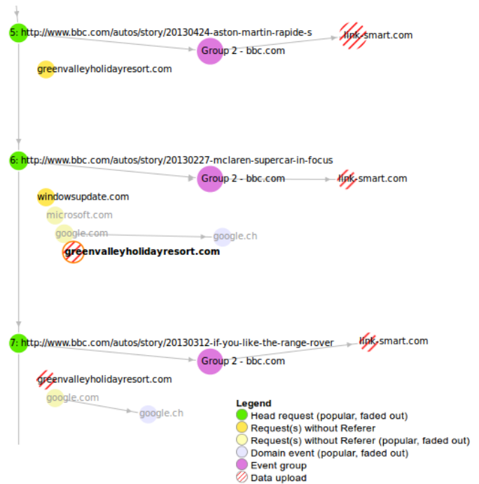
Figure 5: Hviz visualizing Zeus trojan activity taking place during regular Web browsing. The C&C server of this Zeus variant was located at greenvalleyholidayresort.com .
