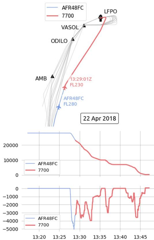
Fig. 14. On April 22nd 2018, Air France flight AFR48FC/AF6127 from Toulouse LFBO to Paris Orly LFPO squawked 7700 as they left the usual STAR procedure route (AMB ODILO VASOL) for a steep descent and a circle to land manoeuvre to landing.
