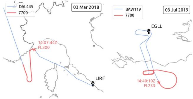
Fig. 9. On March 3rd, 2018, Delta Airlines flight DAL445/DL445 from Rome LIRF to New York KJFK detected an instrument issue when reaching the vicinity of Nice. They turned over the Mediterranean sea to jettison fuel before diverting to Charles-de-Gaulle LFRG. On July 3rd, 2019, British Airways flight BAW119/BA119 bound for Bangalore VOBL interrupted their climb before FL240 and entered into a holding pattern over the Channel to jettison fuel before requesting a priority landing at Heathrow EGLL.
